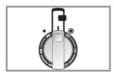
The drawing by each knob indicates which area that knob controls. This one is the right hand dual circuit control.
